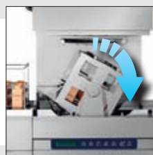
Back rotation for the bottle filling
