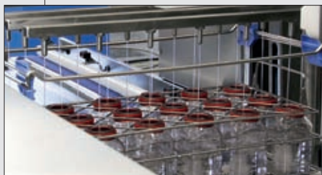
Filling station for two bottle crates
