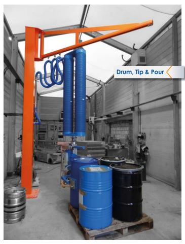
PalPharmaVac<sup>™</sup> - cGMP LIFTING SYSTEMS Ideal for: Transfer of material into and out of application specific containment machines. Handling of active or highly potent compounds where operator protection is an important consideration.
